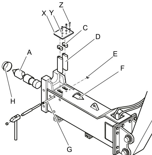
Wiper installed (only hydraulic breakers with DustProtector):
