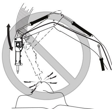
This will damage the hydraulic breaker, the working tool and the carrier.
