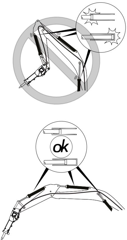
These end positions have damping facilities; the hydraulic cylinder may be damaged by prolonged use while in its end positions.
