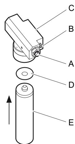
The pump unit (C) must always be sealed to prevent the ingestion of water and dust.
