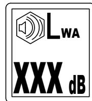
The label states the guaranteed sound power level in accordance with EC directive 2000/14/EC.
