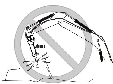
This might cause the working tool to break. Listen to the sound of the hydraulic breaker – it changes when stresses occur between the working tool and the wear bush.
