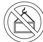
Never lift the hydraulic breaker by the transport safety device. This was not designed for lifting and might break, causing the hydraulic breaker to fall.
