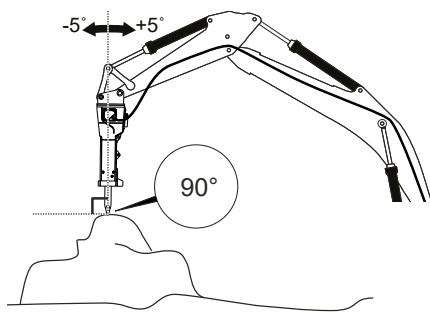
This swing action enables any dust under the tip or the cutter of the working tool to escape. Otherwise a layer of dust is created which would prevent the full percussion energy being transferred to the material to be broken. The tip of the working tool then becomes hot and loses its hardness.
