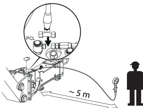
9. Switch on the hydraulic breaker at the lowest possible engine rpm in hydraulic breaker mode.
