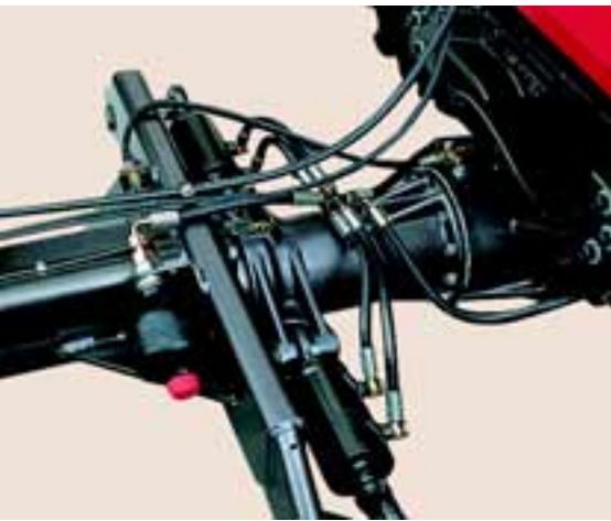
Progressively acting, hydraulic torsion damping between the front and rear axles.
