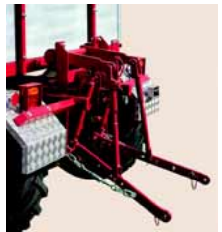
For additional implements: three-point Cat. I and II rear-lifting frame.
