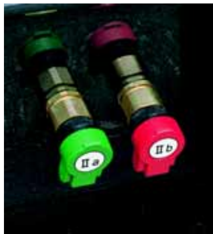
Clearly marked hydraulic connections.
